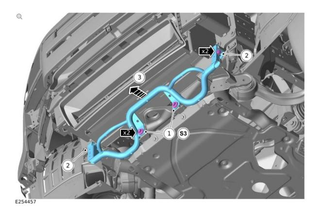
Remove the cooling module protector as illustrated.
