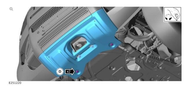
Install, but do not fully tighten the 2 bolts (D) as illustrated.
