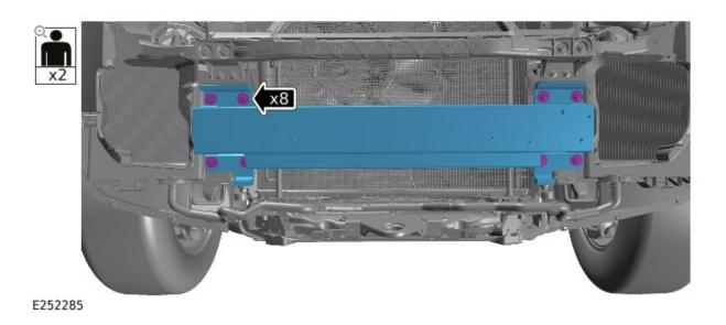
Loosen the 8 armature bolts to assist the installation of the front undershield support bar (A).
