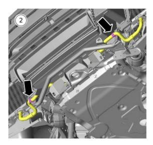
Install the clips (S2) and correctly position the cooling pipe.
