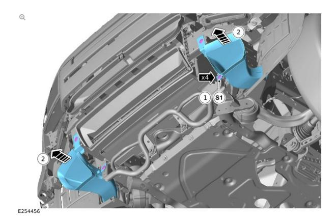
Remove the 2 brake ducts as illustrated. Retain the 4 fixings (S1) that secure the brake ducts to the cooling module protector.
