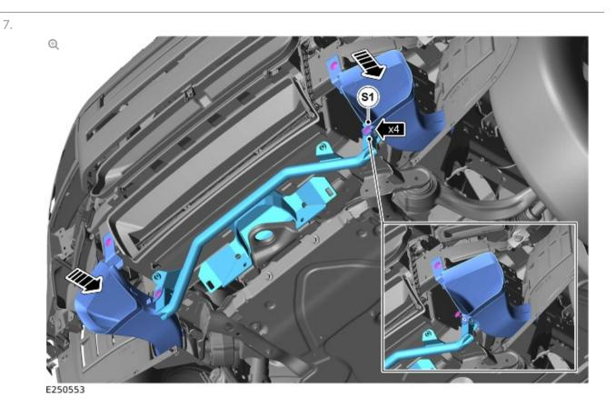
Install the 2 brake ducts to the front undershield support bar using the 4 fixings (S1).
