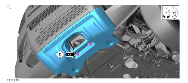
Install, but do not fully tighten the 2 bolts (D) as illustrated.
