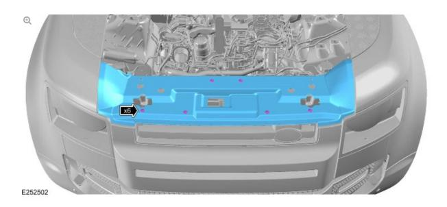
Remove the hood latch panel finisher.
