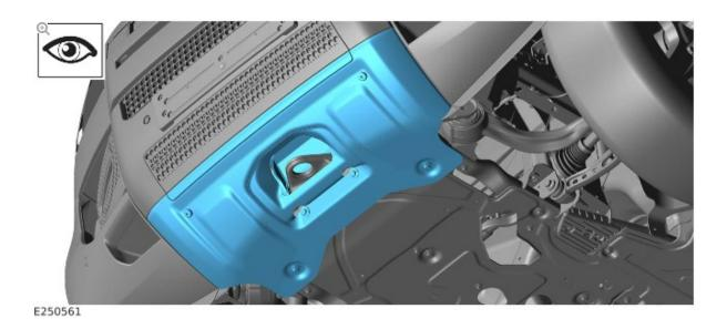
Make sure the front undershield (B) is correctly installed.
