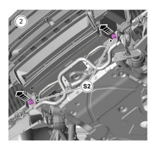
Release and aside the cooling pipe from the cooling module protector as illustrated.
