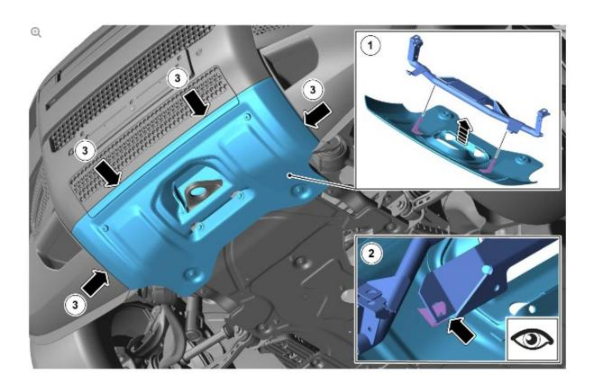
Install the front undershield (B) to the front undershield support bar (A).
