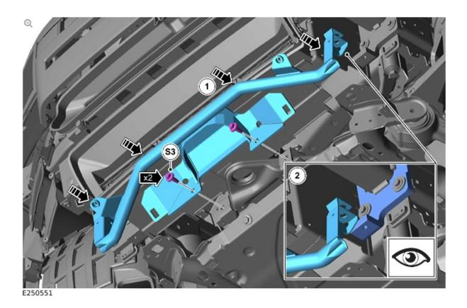
Align and install the front undershield support bar (A).
