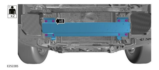
Tighten the 8 armature bolts.
